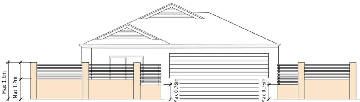
**Figure 2:** Fencing height within the front setback area (as per R-Codes Vol. 1)
